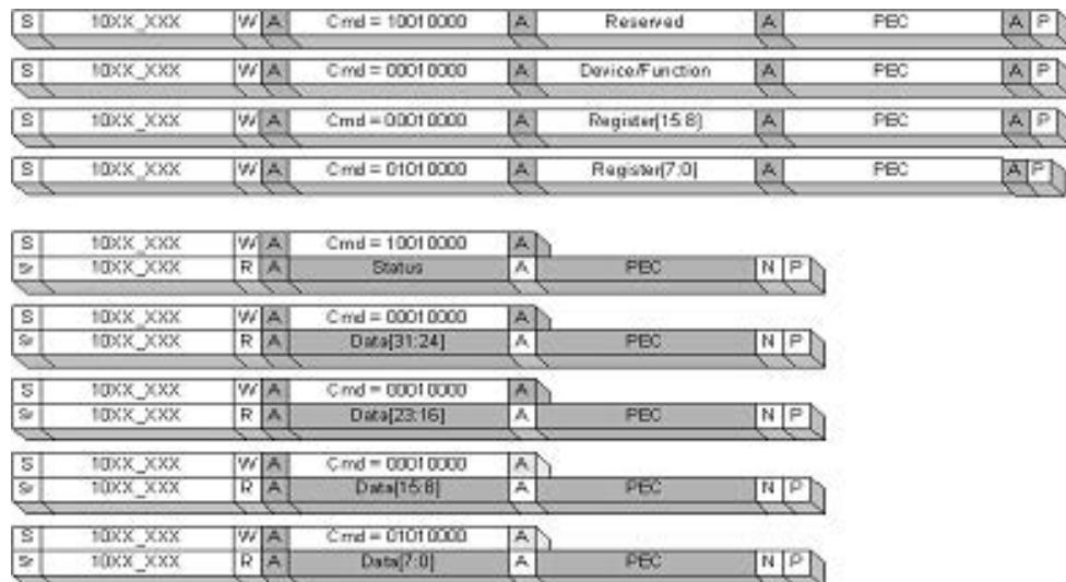
Figure 71 — SMBus Configuration Read (Write Bytes / Read Bytes, PEC Enabled)
